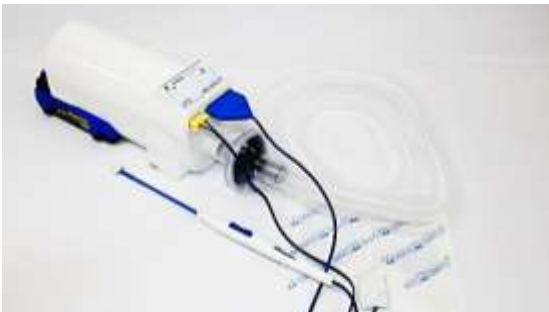
Figure 3: ESU-110 with compatible accessories connected.
