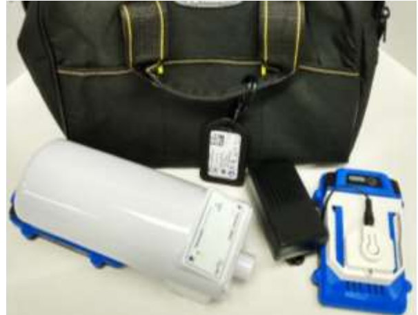
Figure 2: The ESU-110 is battery operated and is designed to be portable.
