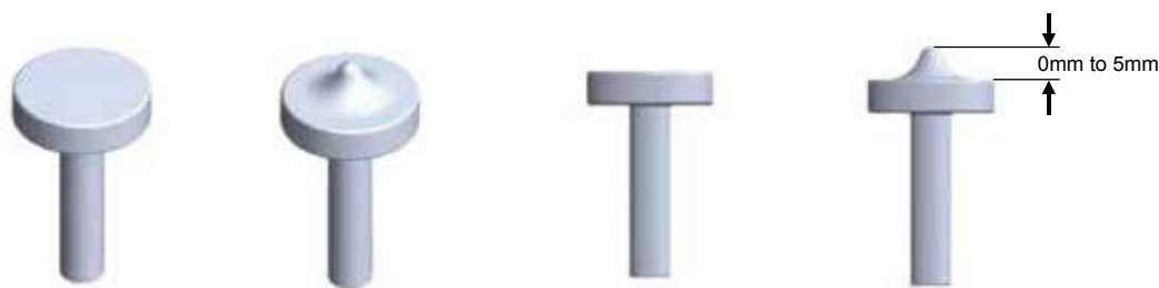
Figure 8.9 Illustration of the cryotips recommended for the treatment of precancerous lesions. Adapted from the WHO technical specifications, 2012. 16
